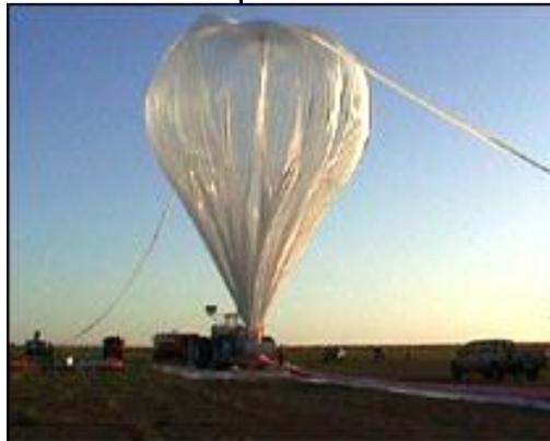
Orbital Payload (AESOP) and Low Energy Electrons (LEE) to observe cosmic rays. The latter alone weighed 1,500 pounds (690 kgs). It is 50 percent more voluminous than standard NASA research balloons, which are 40 million cubic feet (1.1 million cubic meters) in volume and could hold two 747 aircrafts back-to-back inside. Like previous scientific flights, the unmanned balloon, once the tests were finished, was ordered by radio command to drop its experimental payload, which drifted
